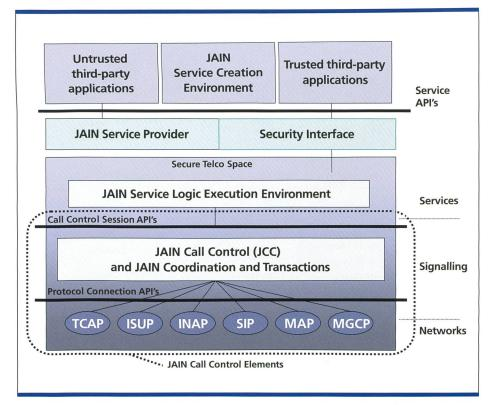
Fig. 4. The JAIN (Java API's for Integrated Networks) environment allows JAIN Trusted Third Party Applications to communicate via a Security Interface with the operator's environment. Within the telecom environment, Services and Signalling layers communicate via API's. (TCAP: Transaction Capabilities Application Part; ISUP: ISDN User Part; INAP: Intelligent Network Application Part; SIP: Session Initiation Protocol; MAP: Mobile Application Protocol; MGCP: Media Gateway Control Protocol).
