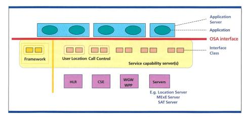
Fig. 3. Open Service Access (OSA) defines an OSA-interface. Applications running on servers located outside the mobile operator domain communicate via this interface. (CSE: CAMEL Service Environment; WGW: Wireless Application Protocol Gateway; WPP: Wireless Application Protocol Push Proxy; MEXE: Mobile Station Execution Environment; SAT: SIM [Subscriber Identity Module] Application Toolkit).
