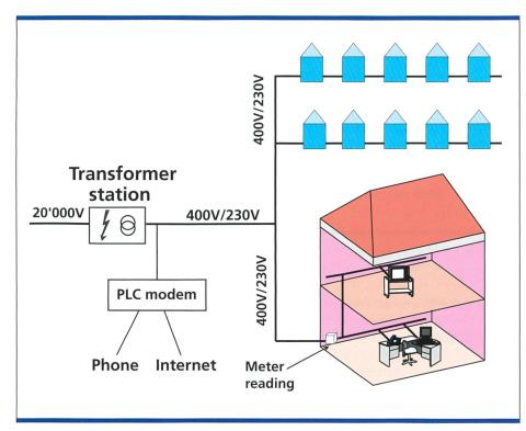
Fig. 3. Installation of a PowerLine modem.
