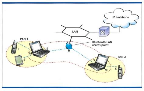
Fig. 12. A scatternet with three interconnected piconets, in which two are PANs and one is used to provide network access to the two PANs via a Bluetooth LAN access point. In this scenario, the letters M and S indicate the distribution of master and slave units.
