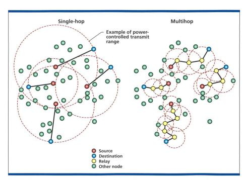
Fig. 9. Comparison of multihop networking with single-hop networking. Both examples have an identical distribution of network nodes.
