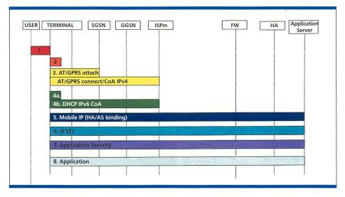
Fig. 3. A message exchange occurs when the GPRS terminal is switched on. The Mobile Internet Service Provider (ISPm) provides Internet connectivity for the GPRS user, while the Firewall (FW) is the boundary between the Internet and a corporate Intranet containing a Home Agent (HA) and Application Server. As a result of the above procedure, Moebius GPRS users can access corporate Intranets in a secure manner with macro-mobility provided by Mobile IP.
