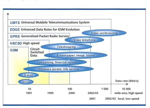
Fig. 4. Evolution of available bandwidth and potential services: Services shaped for 2.5G networks will also be relevant to 3G mobile networks with improved service delivery, end-user devices and interfaces.
