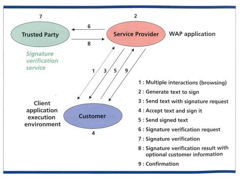
Fig. 5. Verification service for client digital signature.
