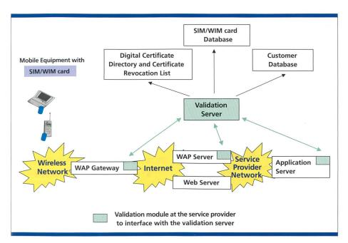
Fig. 3. Overall picture with the required elements.
