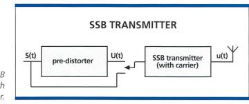
Fig.1. SSB transmitter with pre-distorter.
