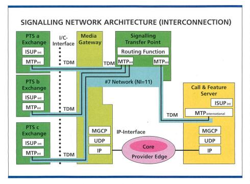
Bild 9. Signalling Network Architecture Interconnection.
