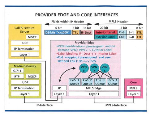
Bild 6. Provider Edge and Core Interfaces.
