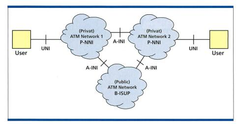
Bild 4. A-INI. User Network Interface; A-INI: ATM Inter-Network Interface; P-NNI: Private Network Node Interface; B-ISUP: Broadband ISDN User Part; ISDN: Integrated Services Digital Network.
