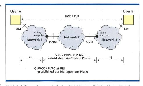
Bild 3. Soft Connections innerhalb eines P-NNI-Netzes. UNI: User Network Interface; P-NNI: Private Network Node Interface; PVC: Permanent Virtual Channel; PVP: Permanent Virtual Path; PVCC: Permanent Virtual Channel Connection; PVPC: Permanent Virtual Path Connection; PVCL: Permanent Virtual Channel Link; PVPL: Permanent Virtual Path Link.
