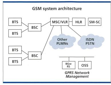
Bild 1. GSM system architecture.
