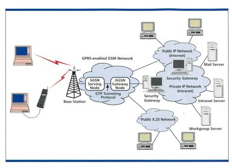
Bild 2. GPRS-Netzstruktur. GSM: Global System for Mobile Communications; GPRS: General Packet Radio Services; IP: Internet Protocol; SGSN: Serving GPRS Support Node; GGSN: Gateway GPRS Support Node; GTP: GPRS Tunnel Protocol.
