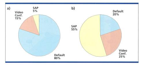
Fig. 2. Typical traffic distribution a) without and b) with policy enforcement at the customer site.
