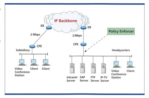
Fig. 1. Typical configuration of a LAN-Interconnect service. The LAN of the head-quarters with a server farm is connected to the LAN of one or more subsidiaries. The dashed line indicates where a policy enforcer can be introduced. ER: Edge Router, CPE: Customer Premises Equipment.
