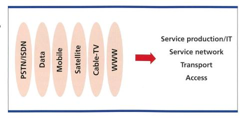
Fig. 1. Paradigm shift from dedicated service networks towards a layered architecture with common network technologies. Currently, there are separate network technologies as shown on the left, but in future this is expected to change.
