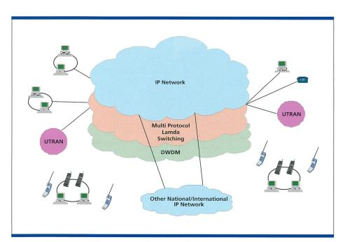
Fig. 6. Future Unified Fixed/Mobile Network? IP-services are supported by MPLS currently implemented in the Swisscom IP-backbone network. The IP network is connected over Multi Protocol Lamda Switching to DWDM (Dense WDM).
