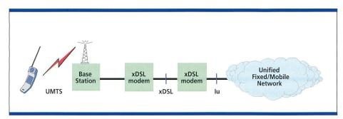
Fig. 4. Alternatively, xDSL is connected directly to an lu-compliant core network which handles both circuit-switched and packet traffic. The core network is the "Unified Fixed/Mobile Network".
