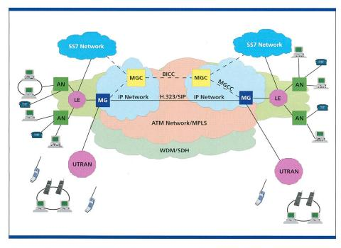
Fig. 5. In this scenario, SS7 signalling trunks from the national/international telephony networks are connected to Media Gateway Controllers, while voice trunks are terminated at Media Gateways. An ATM/MPLS core network is supported by WDM/SDH and the Bearer Independent Call Control protocol is used between Media Gateways Controllers.
