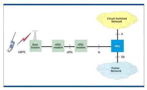
Fig. 3. Fixed network evolution towards UMTS. The copper local loop has been upgraded to xDSL. A UMTS base-station providing cordless access has been added at the customer premises. At the operator side, an Inter-working Unit (IWU) separates circuit-switched and packet traffic into respective (legacy) networks in similar manner to figure 2.
