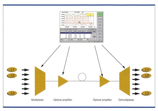
Fig. 3. Testing with a multiwavelength meter.
