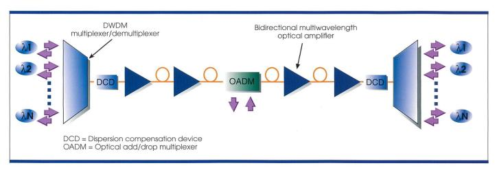
Fig. 1. DWDM optically amplified system.
