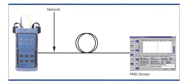
Fig. 2. Testing PMD.
