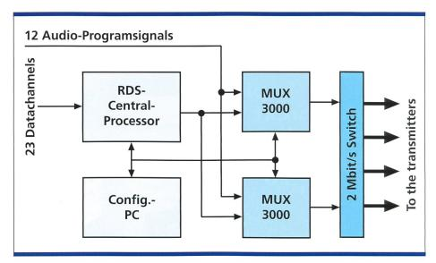
Fig 1. Old feeding principle.
