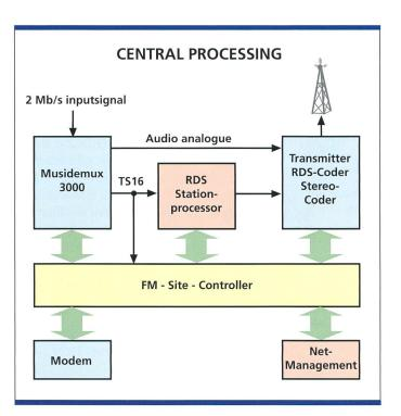
Fig 6. G.703 MO-DAT-ensemble; shortcuts for different programsignals.
