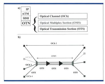
Fig. 3a. Schematics of a network with IP/ATM/SDH over the OTN, showing the ITU-T three layer model for the OTN.
