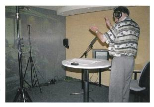
dual microphone set up. The dual microphone was placed next to the video wall. For both systems a matrix was used for the correct three dimensional reproduction of the sound.
