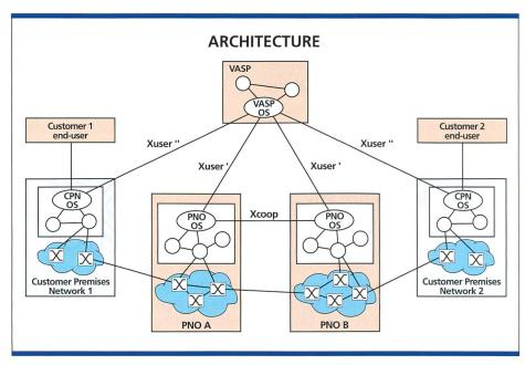
Fig. 1. The TRUMPET Reference Architecture.
