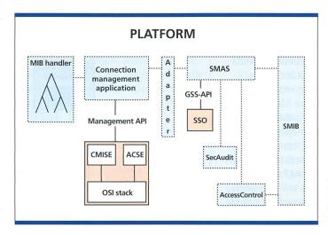
Fig. 2. Architecture for a Commercial Management Platform
