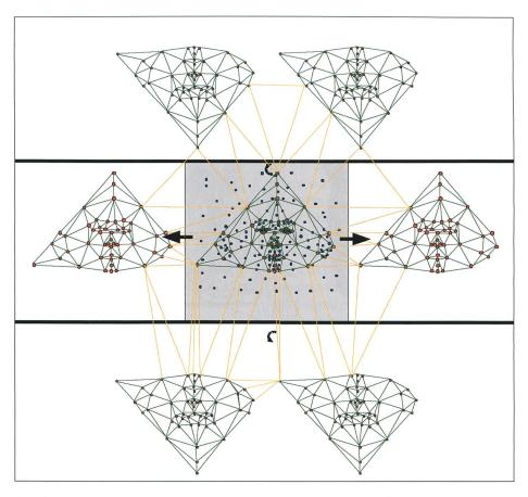
Fig. 6. Expansion of the feature points – Linked dots: Projected feature points – Unlinked dots: Projected non-feature points – Dark lines: Feature points triangulation – Light lines: Expanded triangulation.
