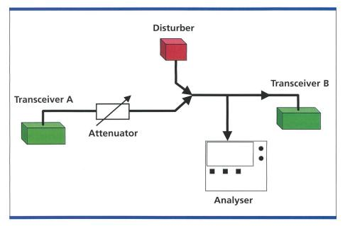
Fig. 5. Cable bound simulation of the EMC situation of figure 4. The attenuator simulates propagation loss.
