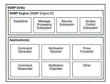
Fig. 1. An SNMP Entity and its components
