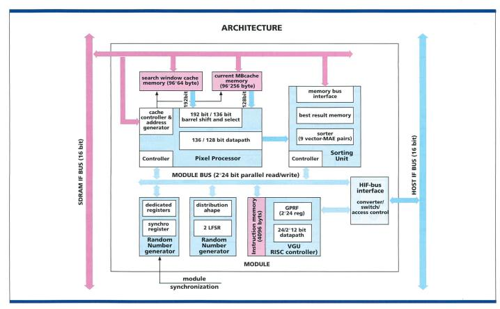
Fig. 4. Architecture of one module.
