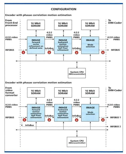
Fig. 5. Encoder configuration examples using the image chip.
