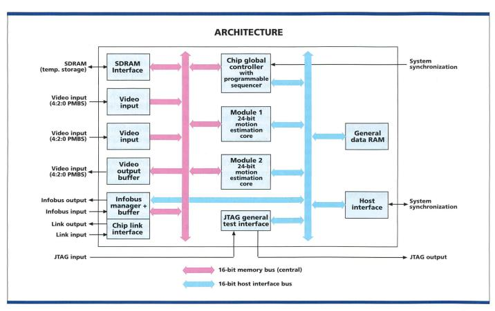
Fig. 3. Image chip architecture.
