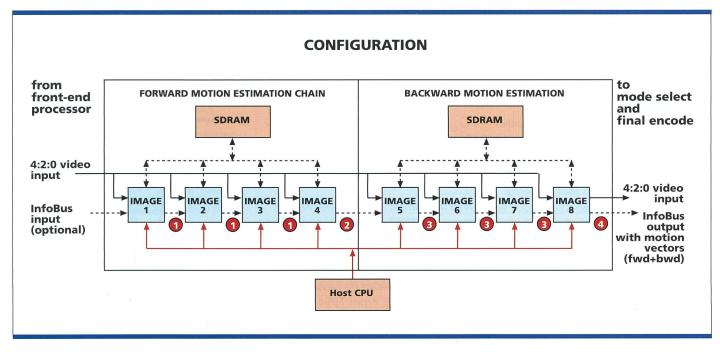
Fig. 6. Image multi-chip configuration example (increase of the search window to 192¥128 pixel). Tab. 1. Image chip features.
