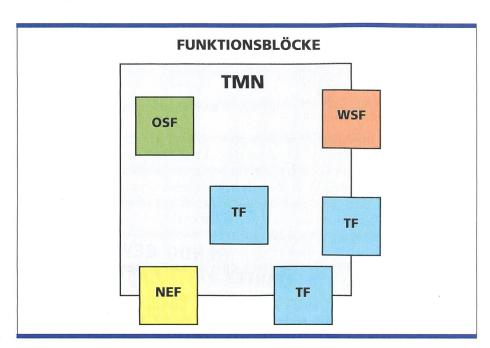
Bild 1. TMN-Funktionsblöcke [draf rec. ITU-T M.3010/M.3013 (1999)]. TMN Functional Blocs: OSF: Operation System Function, TF: Transformation Function, WSF: Work Station Function, NEF: Network Element Function.
