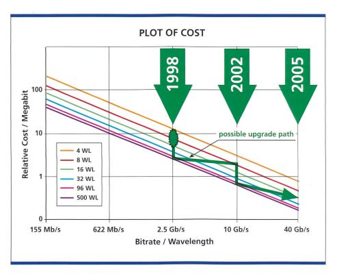
Fig. 5. Plot of cost per transmitted Megabit as a function of the bitrate per wavelength and the number of wavelengths.
