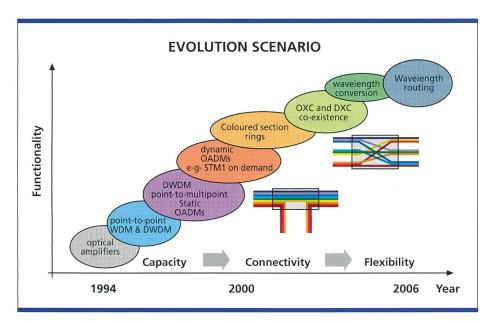
Fig. 6. Evolution scenario from amplified WDM point-to-point links to a wavelength routed network layer.
