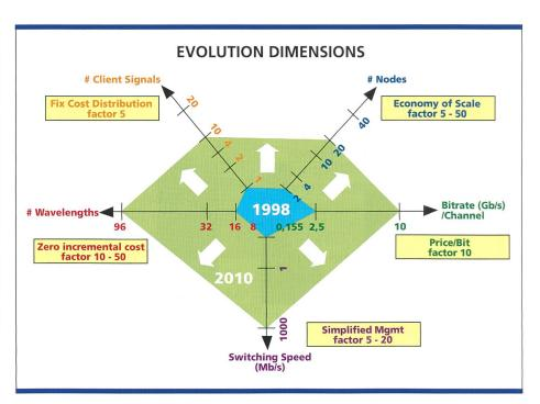
Fig. 4. Evolution dimensions in optical networking and potential cost saving factors. Please note that the indicated dimensions are not independent and, hence, neither are the given cost reduction factors.
