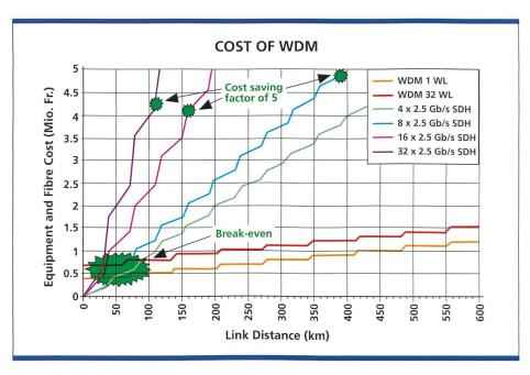
Fig. 1. Cost of WDM based transmission systems vs. systems based on parallel fibres as a function of the link length and the number of parallel systems (corresponding to the number of wavelengths).
