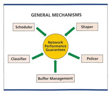
Fig. 1. General mechanisms for offering network performance guarantees: Classifiers, policers, buffer management mechanisms, schedulers and shapers are the building blocks for offering network performance guarantees.
