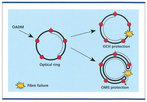
Fig. 3. Optical channel protection and optical multiplex-section protection.
