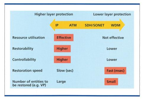
Fig. 2. Characteristics of each layer protection.
