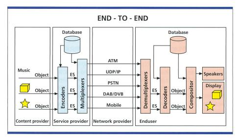
Fig. 1. End-to-end connection, conceptual diagram.
