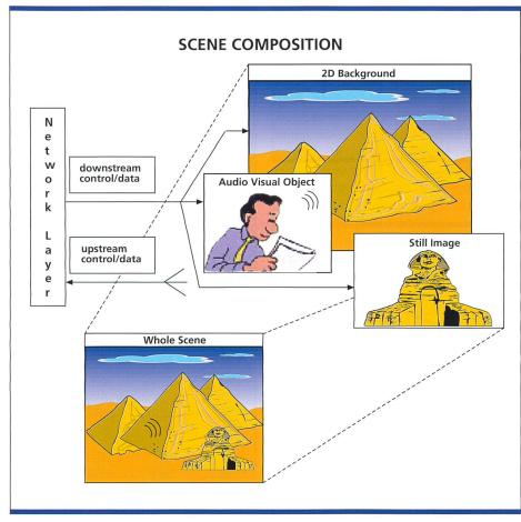
Fig. 10. The composition of an MPEG-4 scene.
