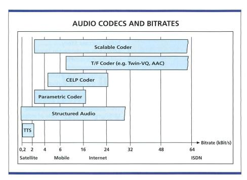
Fig. 3. The MPEG-4 audio codecs and the corresponding bitrate per channel.
