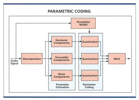
Fig. 4. MPEG-4 Parametric codec block diagram.
