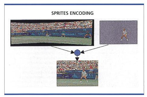
Fig. 8. Encoding of background pictures with sprites.
