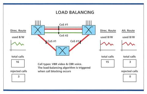
Fig. 4. Dynamic load balancing.
