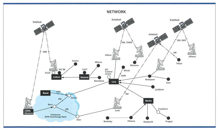
Fig. 8. The Network Scenario for the IDC '98 Conference (host site Lisbon) (links are 4 Mbit/s ATM, except where indicated otherwise).
