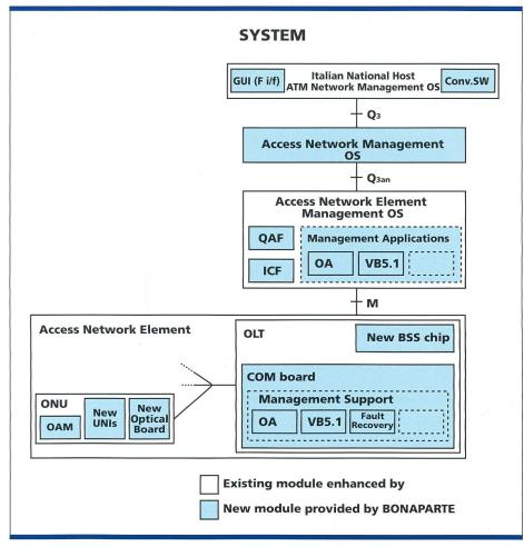
Fig. 2. Enhancements of the existing system.
