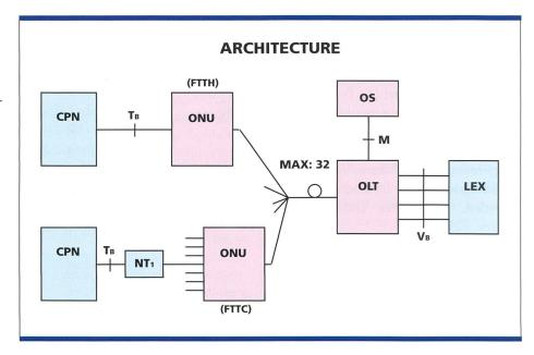
Fig. 1. Architecture of the existing access network.
