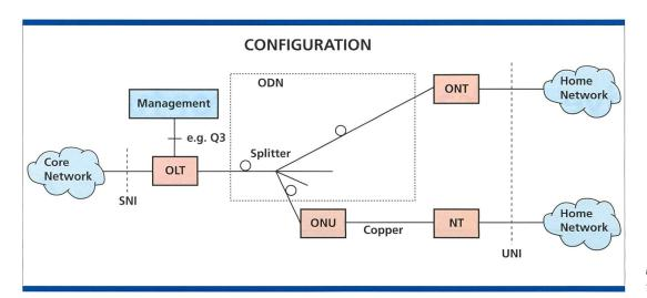
Fig. 1. Basic configuration of an APON.
