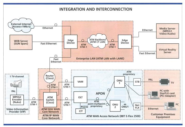
Fig. 5. APON integration and interconnection in the laboratory. The ATM/SDH WAN is represented in the laboratory by an ATM switch, the ATM/IP WAN by an ATM switch and a router. A video information provider is represented by a PAL TV channel and a MPEG2 encoder. The ATM based enterprise LAN can be interpreted as the LAN of a business customer, to which the PCs (residential customers) connected to the APON can set-up connections e.g. for teleworking.
