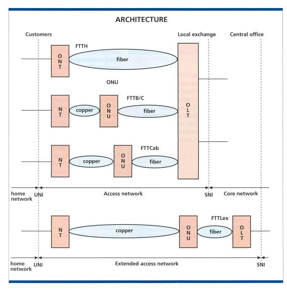
Fig. 2. Network Architecture using APONs.
