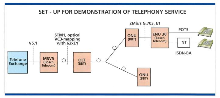
Fig. 6. Set-up for the demonstration of telephony service in the laboratory with multiplexing equipment available from Bosch Telecom. The STM1 signal at the OLT is demultiplexed to a V5.1 signal by the MSV5 multiplexer which can be connected to the telephone exchange. On the ONU side, the ENU30 multiplexer, to which the telephones and ISDN network terminations (NTs) can be connected, demultiplexes the E1 G.703 signal to POTS and ISDN-BA signals.
