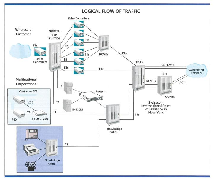
Figure 5. The network diagram shows the logical flow of traffic from the customer's premises into SCNA's international point of presence (I-PoP) and from there to Switzerland or any place in the world.
