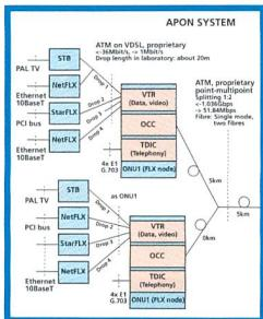
ATM passive optical networks (APONs) are foreseen to be one of the most cost effective fiber-based solutions for broadband access networks. They allow a flexible bandwidth allocation to customers, and can be installed in different architectures, ranging from "fiber to the local exchange" to "fiber to the home," using the same type of equipment.
