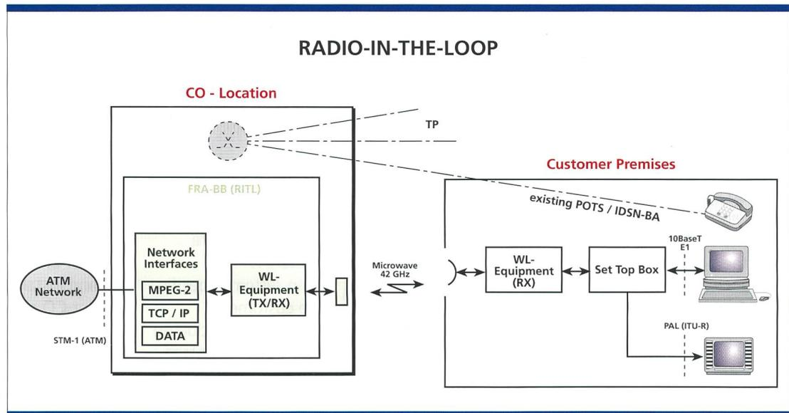
Figure 5. Radio-In-The-Loop (RITL): Fixed Radio Access-BroadBand (FRA-BB) principle.
