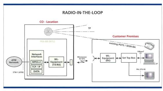
Figure 5. Radio-In-The-Loop (RITL): Fixed Radio Access-BroadBand (FRA-BB) principle.
