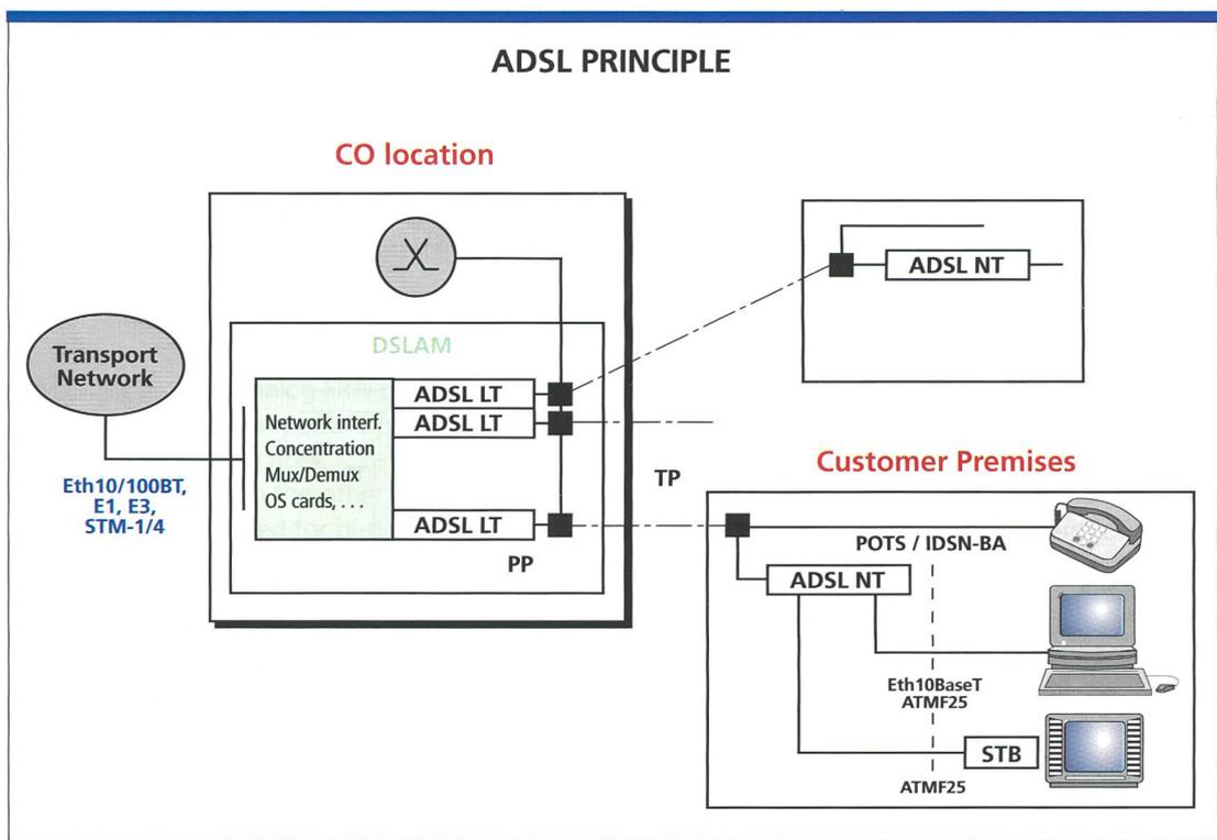
Figure 3. ADSL principle.
