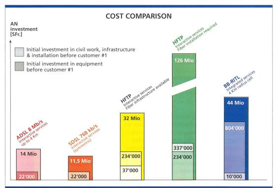
Figure 6. Cost comparison between different technical solutions for the delivery of NB and BB interactive services (simplified model).
