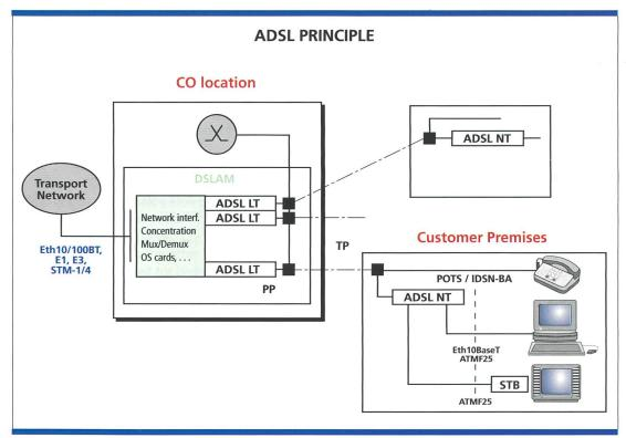
Figure 3. ADSL principle.
