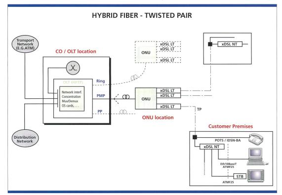
Figure 4. Hybrid Fiber-Twisted Pair (HFTP) principle.
