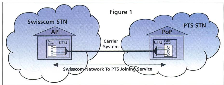
**Figure 1.** The service allows connection of the Swisscom and Provider of Telecommunications Services networks for the exchange of signalling messages and to allow calls to be passed between Swisscom and the Provider of Telecommunications Services (Fig. 1). This service or an equivalent service supplied by the Provider of Telecommunications Services is necessary to support the other services in the Swisscom portfolio.
