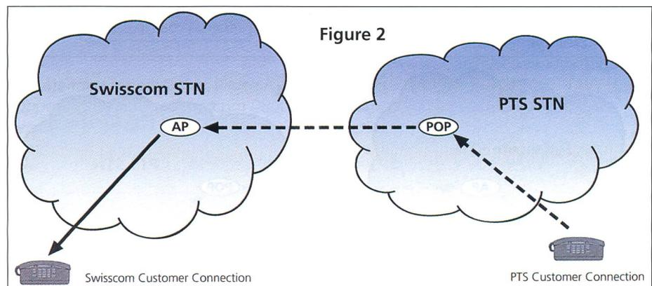
**Figure 2.** Many new entrants will want to deliver calls to existing Swisscom telephone connections. This service allows new entrants to make universal service calls available to Swisscom at an Access Point for delivery to the destination Swisscom telephone connection, enabling the Provider of Telecommunications Services to offer "any to any" services to its own customers.
