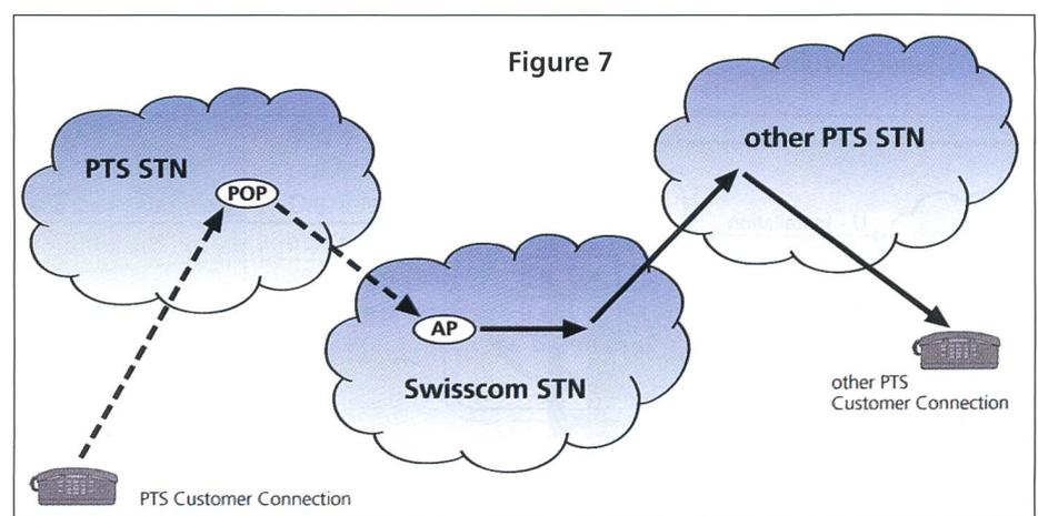
PoP = Point of Presence = A PTS location which is offered for connection to exactly one Swisscom Access Point in the same access area, which is part of the PTS switched telecommunications network and is within the geographic area of Switzerland in which the PTS is
