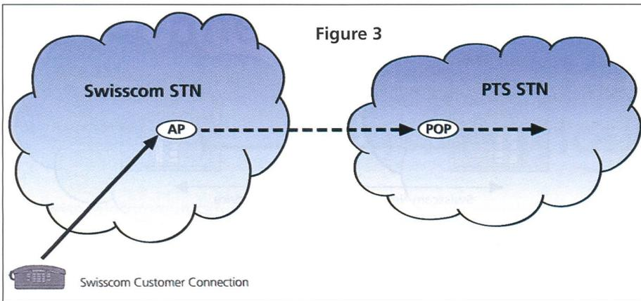
**Figure 3.** Users of telecommunications services in Switzerland now have the possibility to choose a carrier for their universal service calls. Their selection is indicated by use of a short code which is used before the full telephone number is dialled. This service allows users of Swisscom fixed telephones to select a Provider of Telecommunications Services to carry a call, allowing reach from Swisscom's current customers.
