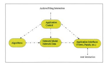
Fig. 1. Basic components of a network planning and optimization application.
