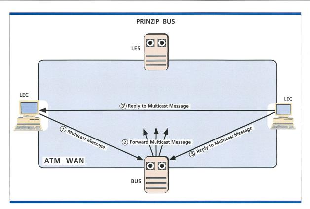
Bild 6. Prinzip des Broadcast Unknown Servers (BUS). LEC: LAN Emulation Client, BUS: Broadcast Unknown Server, LES: LAN Emulation Server, LE-ARP: LAN Emulation Address Resolution Protocol, VCC: Virtual Channel Connection, VCI: Virtual Channel Identifier, MAC: Medium Access Control.
