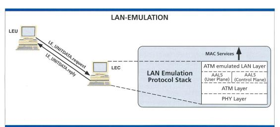
Bild 3. LAN Emulation Protocol Stack. MAC: Medium Access Control, LEU: LAN Emulation User, LEC: LAN Emulation Client, AAL: ATM Adaptation Layer.
