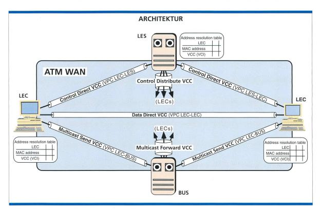
Bild 4. Architektur für LAN-Emulation (Kommunikationsinfrastruktur). LES: LAN Emulation Server, LEC: LAN Emulation Client, BUS: Broadcast Unknown Server, LE-ARP: LAN Emulation Address Resolution Protocol, VCC: Virtual Channel Connection, VCI: Virtual Channel Identifier, MAC: Medium Access Control.
