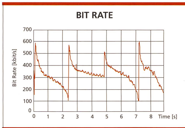
Fig. 2. Bit rate of a 'lossless coder' (uncompressed bit rate: 705.6 kbit/s).
