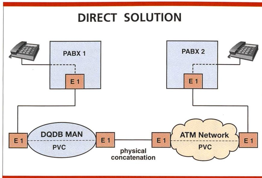
Fig. 2. MAN/ATM: direct solution.
