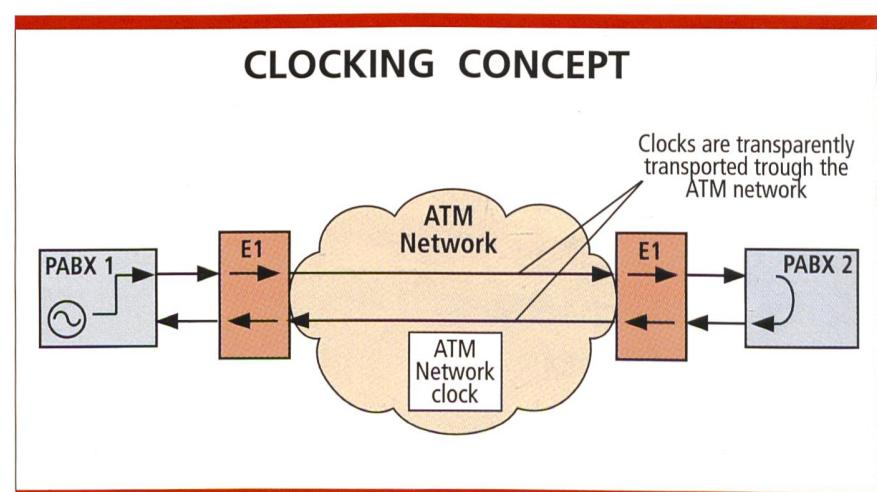
Fig. 1. Plesiochronous clocking concept with master-slave PABXs.
