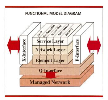
Bild 28. Functional Model Diagram. Management Areas: F = Fault Management, C = Configuration Management, A = Accounting Management, S = Security Management; Management Layers: BML = Business Management Layer, SML = Service Management Layer, NML = Network Management Layer, EML = Element Management Layer.
