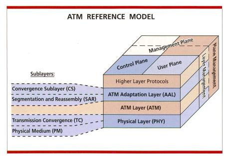
Bild 1. ATM Reference Model: Layers, Sublayers and Planes.
