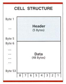
Bild 2a. Cell Structure at NNI and UNI [ITU-T I.361].
