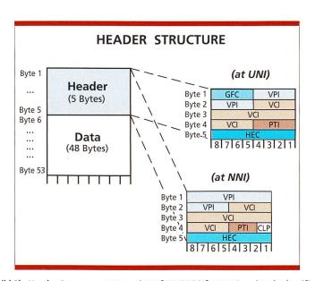
Bild 2b. Header Structure at NNI and UNI [ITU-T I.361]. VPI: Virtual Path Identifier, VCI: Virtual Channel Identifier, GFC: Generic Flow Control, PTI: Payload Type Identifier, CLP: Cell Loss Priority, HEC: Header Error Check, NNI: Network Node Interface, UNI: User Network Interface.
