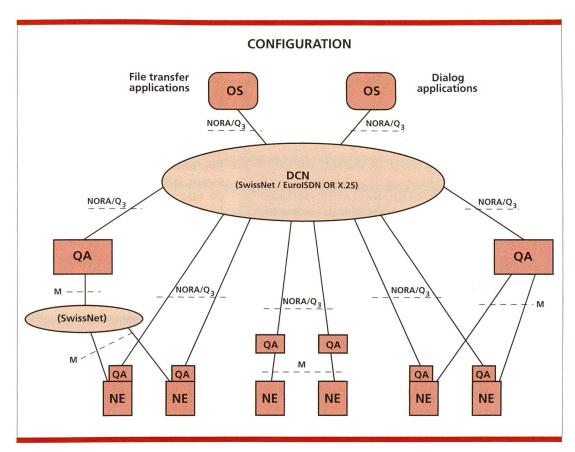
Fig. 5. Short-term target configuration.
