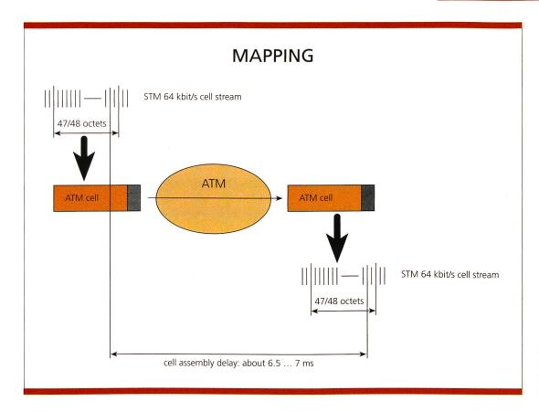
Fig. 3. Mapping of 64-kbit/s cell stream onto ATM.
