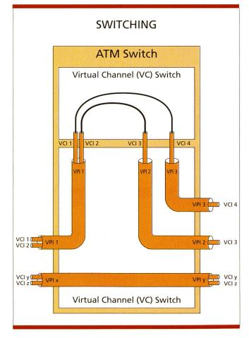
Fig. 1. ATM VP/VC switching.
