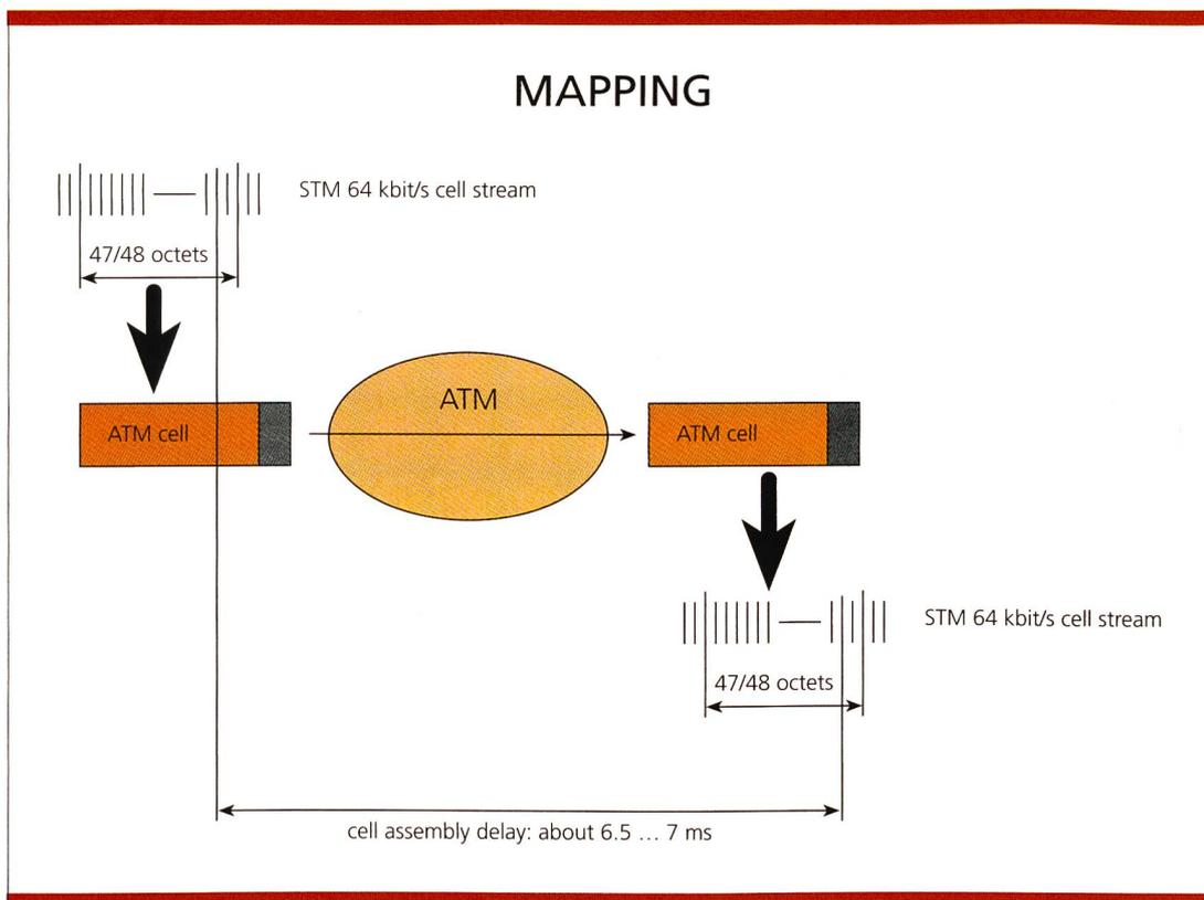
**Fig. 3. Mapping of 64-kbit/s cell stream onto ATM.**
