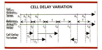
Fig. 2. Illustration of cell delay variation.
