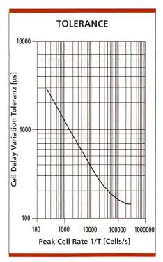
Fig. 5. Cell delay variation tolerance at the input of the Swiss ATM network in function of the peak cell rate (provisional values).
