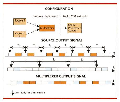
Fig. 1. Multiplexing of the cell streams of two ATM sources, presenting cells at constant time spacings.
