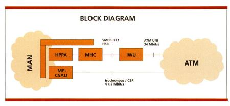
Fig. 4. IWU block diagram.
