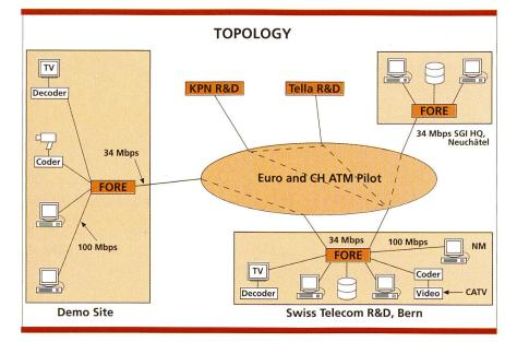
Figure 2. Topology of the ATM Xorporate Networks platform.
