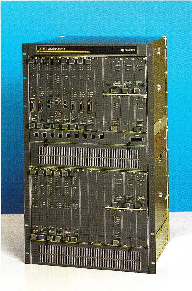
Fig. 2. Service multiplexer 36150 in the redundant 8-portrack Version
