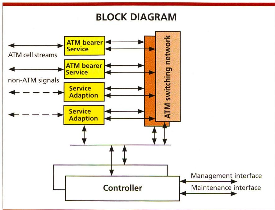
Fig. 1. Block diagram of a service multiplexer.
