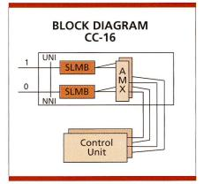
Fig. 2 Block diagram of an ATM cross-connect ATM-CC-62/16. SLMB: Subscriber Line Module Broadband; TMB: Trunk Module Broadband; UNI: User Network Interface; ASN: ATM Switching Network; AMX: ATM-Multiplexer (ATM-Max); NNI: Network Node Interface.
