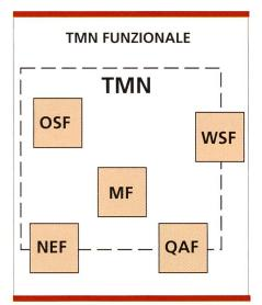
Fig. 1a. Architettura TMN funzionale (M.3010). OSF: Operation System Function; MF: Mediation Function; WSF: Work Station Function; NEF: Network Element Function; QAF: Q Adaptor Function.
