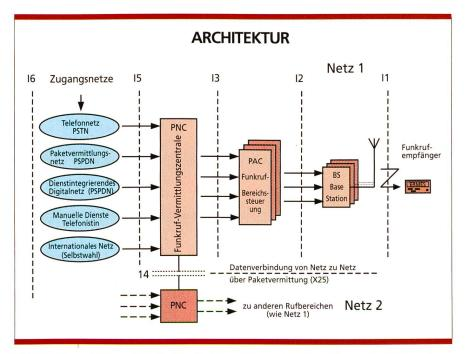
Bild 2. Systemarchitektur. I1 bis I6: Schnittstellen, PNC: Paging Network Controller, PAC: Paging Area Controller, PSTN: Public Switched Telephone Network, PSPDN: Packet Switched Public Data Network, ISDN: Integrated Services Digital Network.
