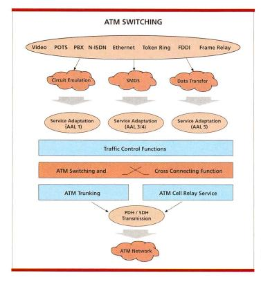
Fig. 1. Sevice adaptation and ATM switching – the cornerstone of the AAU
