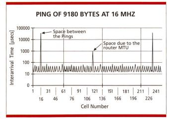
Fig. 1. Interarrival time of the cells during a ping of 9180 Byte at 16 MHz (214 ATM cells). The router is configured with a MTU of 4470 Byte.
