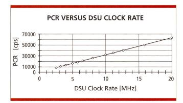
Fig. 9. Peak cell rate versus DSU clock rate.
