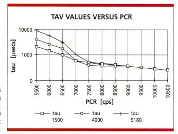
Fig. 6. τ values versus PCR for different ping packet sizes (1500, 4000 and 9180 Byte) and for a DSU clock rate of 2.5 MHz.
